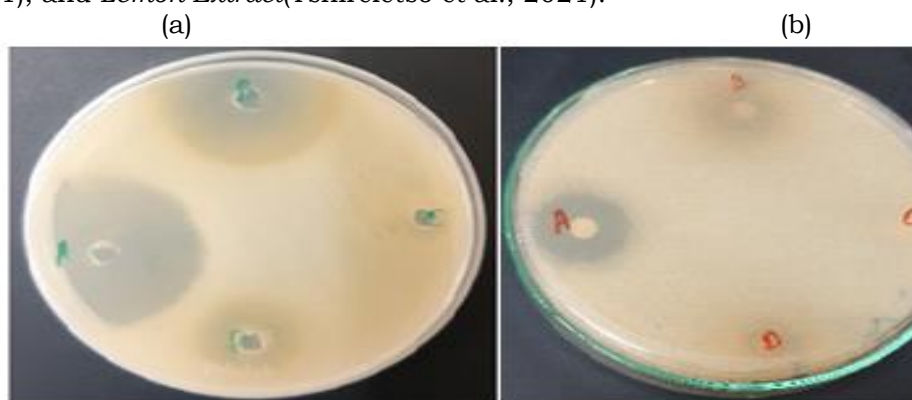
Figure 9. Antibacterial activity of CuONPs against L. monocytogenes : (a) agar well diffusion and (b) disc diffusion technique [Where, A = chloramphenicol, B = CuONPs, C = Plant extract, D = \text{Cu}(\text{NO}_3)_2 ].
