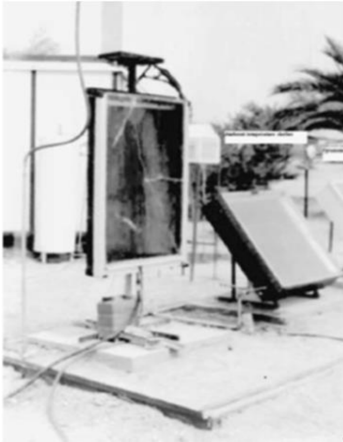
Fig. 16: Photographic view of vertical solar still [30]
