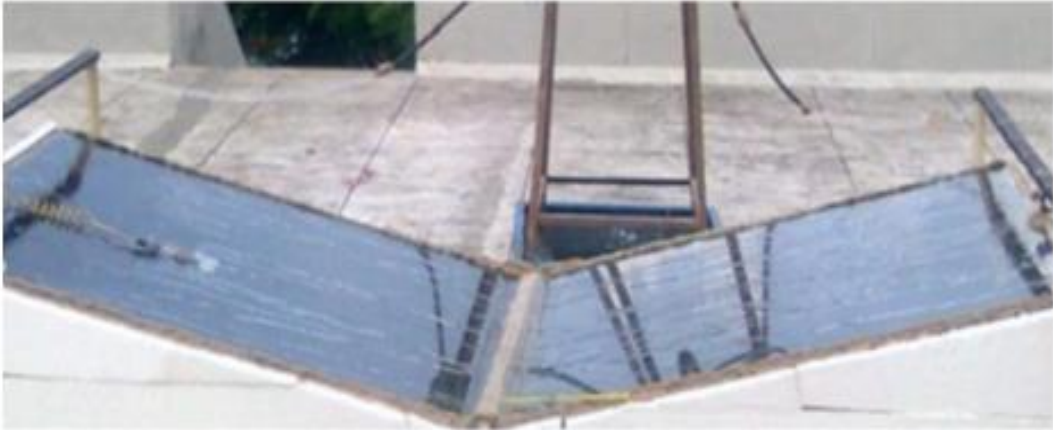
Fig. 18: Top cover cooling arrangement of V type solar still [32]
