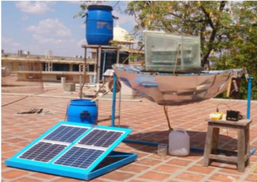
Fig. 13: Photo of the triple basin solar system [28].
