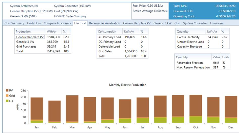
Figure 9. Contribution of various sources of electrical energy to the hybrid system.
