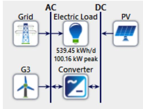
Figure 2. Diagram of a microgrid with integration of renewable energies.
