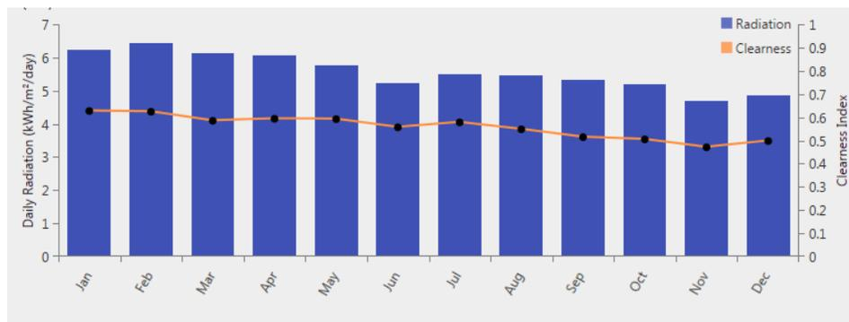
Figure 5. Average radiance values at the proposed site for microgrid installation
