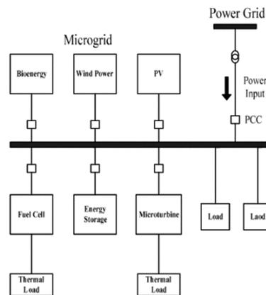
Figure 1. Basic structure of a microgrid
