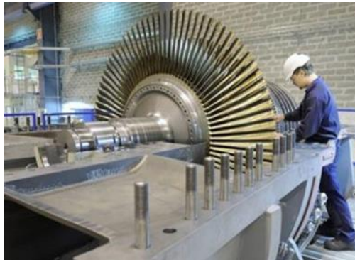
Figure 6. Steam Turbine Source: (Vásquez Calero & Mora Robles, 2016)
