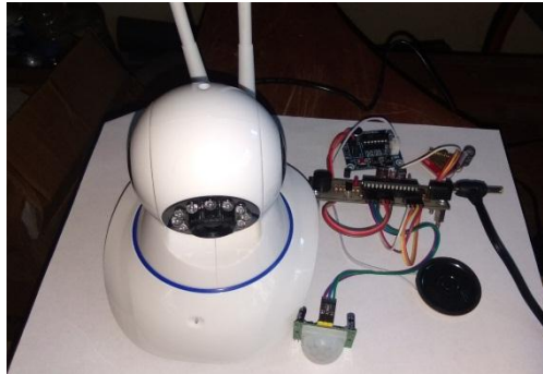
Figure 2. Tool design using PIR sensor and ATmega328 microcontroller to improve online CCTV work
